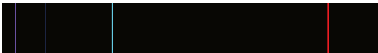
Figure 2.15 The emission spectrum of atomic hydrogen: The spectral positions of emission lines are characteristic for hydrogen atoms. (credit: “Merikanto”/Wikimedia Commons)
