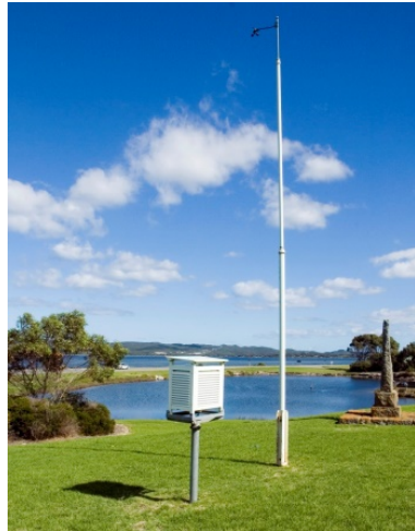
Stevenson screen and anemometer are used to measure weather conditions.
