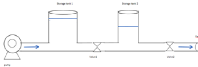
Figure 8-6 A hydraulic system with a pump
