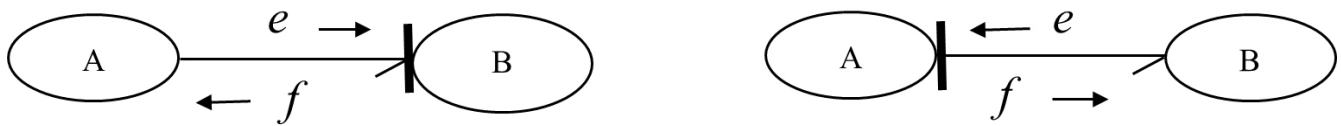
Figure 3-3 Causality assignment definition and directions of effort and flow between elements A and B
