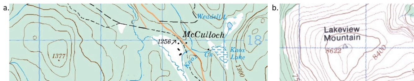
Figure 15.6. a. Example of a spot height (elevation = 1377) and a benchmark (elevation = 1256). b. Example of a horizontal control point (elevation = 8622). Note: Elevation units may be feet or metres – you need to check the map. Sources: a. NTS 1:50,000 map sheet 82E14 (Kelowna) 4th edition. b. NTS 1:50,000 map sheet 92H01 (Ashnola River) 2nd edition. Natural Resources Canada, Open Government License-Canada .
