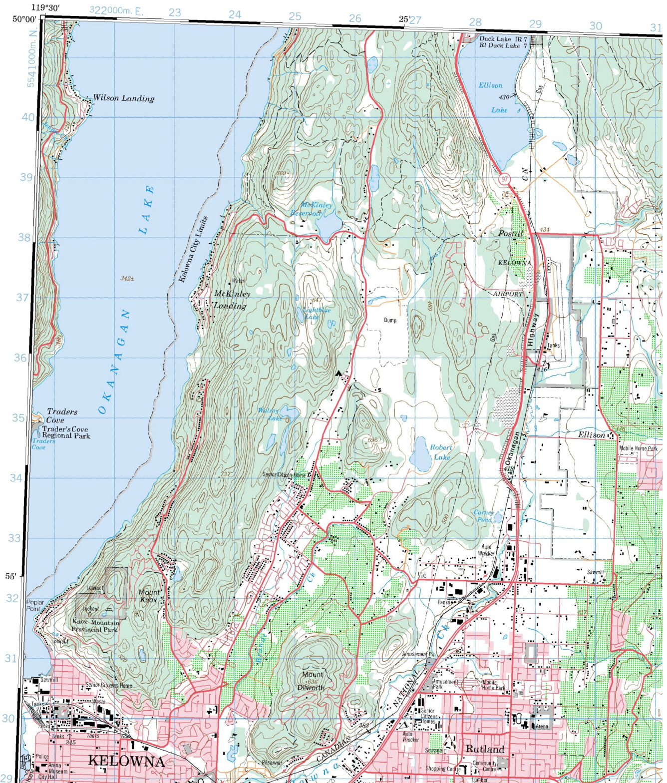
Figure 14.1. Part of NTS 1:50,000 map sheet 82E14 (Kelowna) 4th edition. Notice that in this example, the map's neatlines are tilted slightly, and are not parallel to the blue UTM grid. This area lies within UTM quadrilateral 11U. Source: Natural Resources Canada, Open Government License-Canada . [Click to view image full size]
