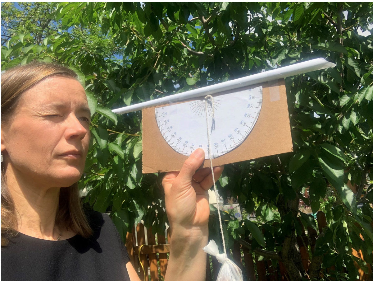
Figure 16.15. Photograph of a level constructed with the protractor template in Appendix B, cardboard, a string with a weight, and rolled paper being used as a sighting tube. Source: C. Huscroft, CC BY-NC-SA 4.0.
