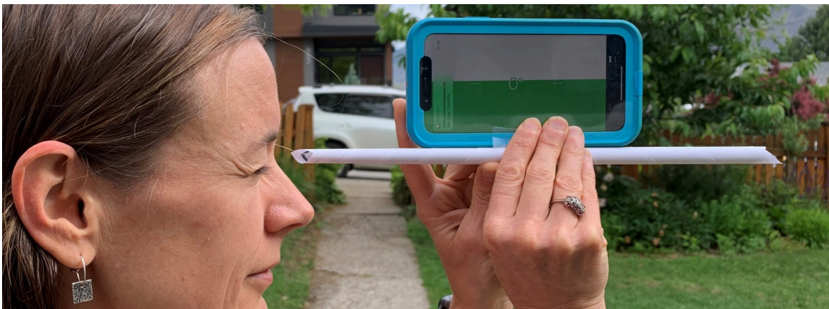
Figure 16.14. Photograph of rolled paper being used as a sighting tube by affixing it with tape to a cell phone. Note that the screen indicates that a reading of 0 degrees has been reached. Source: C. Huscroft, CC BY-NC-SA 4.0.
