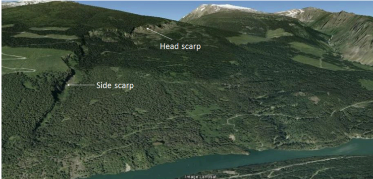
Figure 15.9 The Downie Slide, a sacking, on the shore of the Revelstoke Reservoir (above the Revelstoke Dam). The head scarp is visible at the top and a side-scarp along the left side. [from Google Earth]
