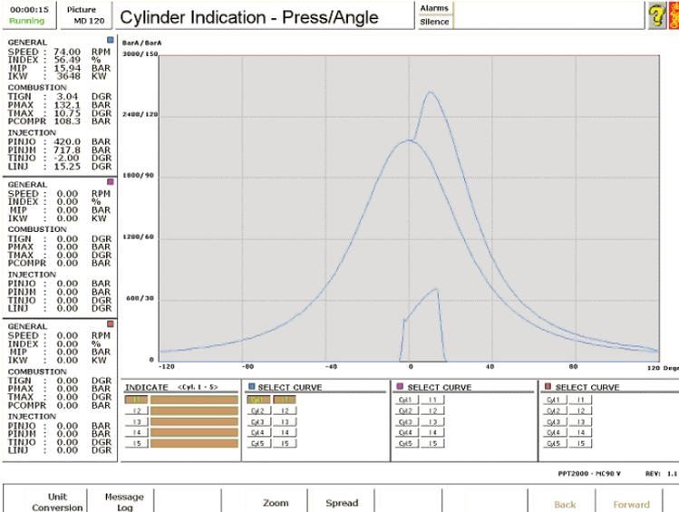
At the instant when the cylinder indicator is taken, the following parameters are displayed on the left hand side, in the numeric data display,
