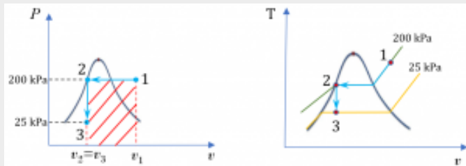
Figure 4.4.e5 P-v and T-v diagrams of the whole process
