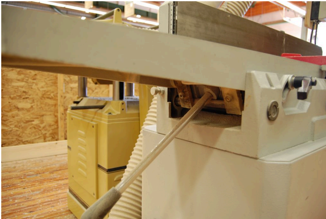
Jointer with pivoting arm adjustments
