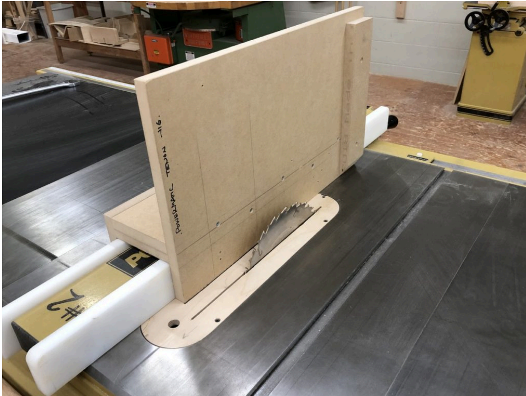
Simple vertical carrier for the T rip fence.
