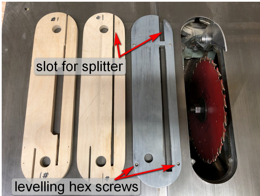
Throat plates, left to right: shop made for dado, shop made, and factory.
