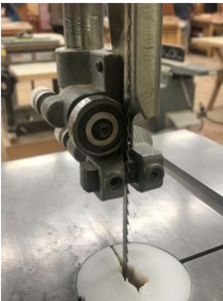
Upper band saw guides, block type
