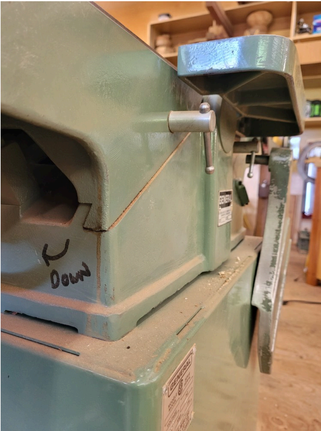
Jointer with dovetail way adjustments
