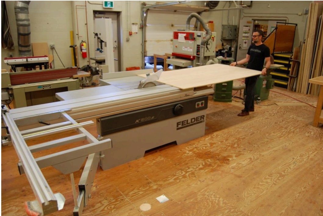
Ripping a full sheet on the panel saw
