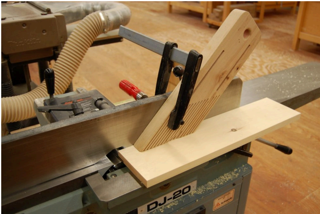
Jointing a face rabbet with a featherboard
