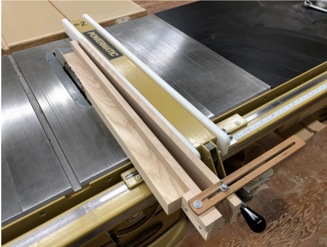
Adjustable taper jig, shown with part in position ready for tapering.
