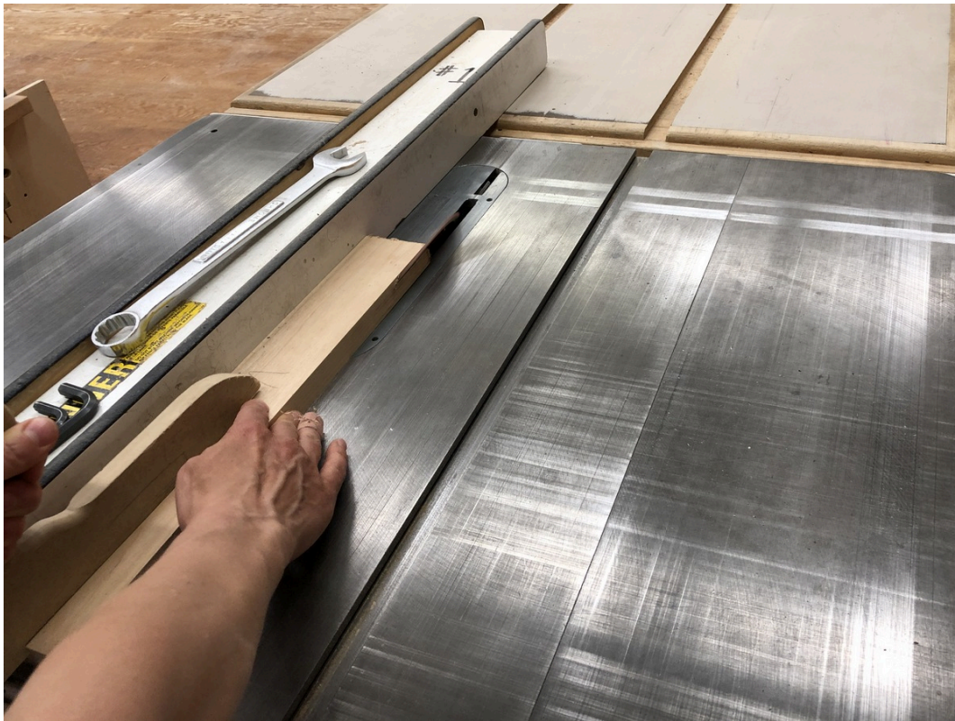
Ripping bevels on a right tilt saw
