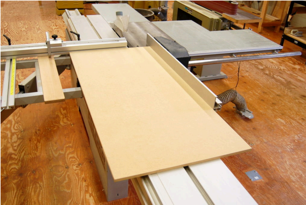
Using the rip and crosscut fence together
