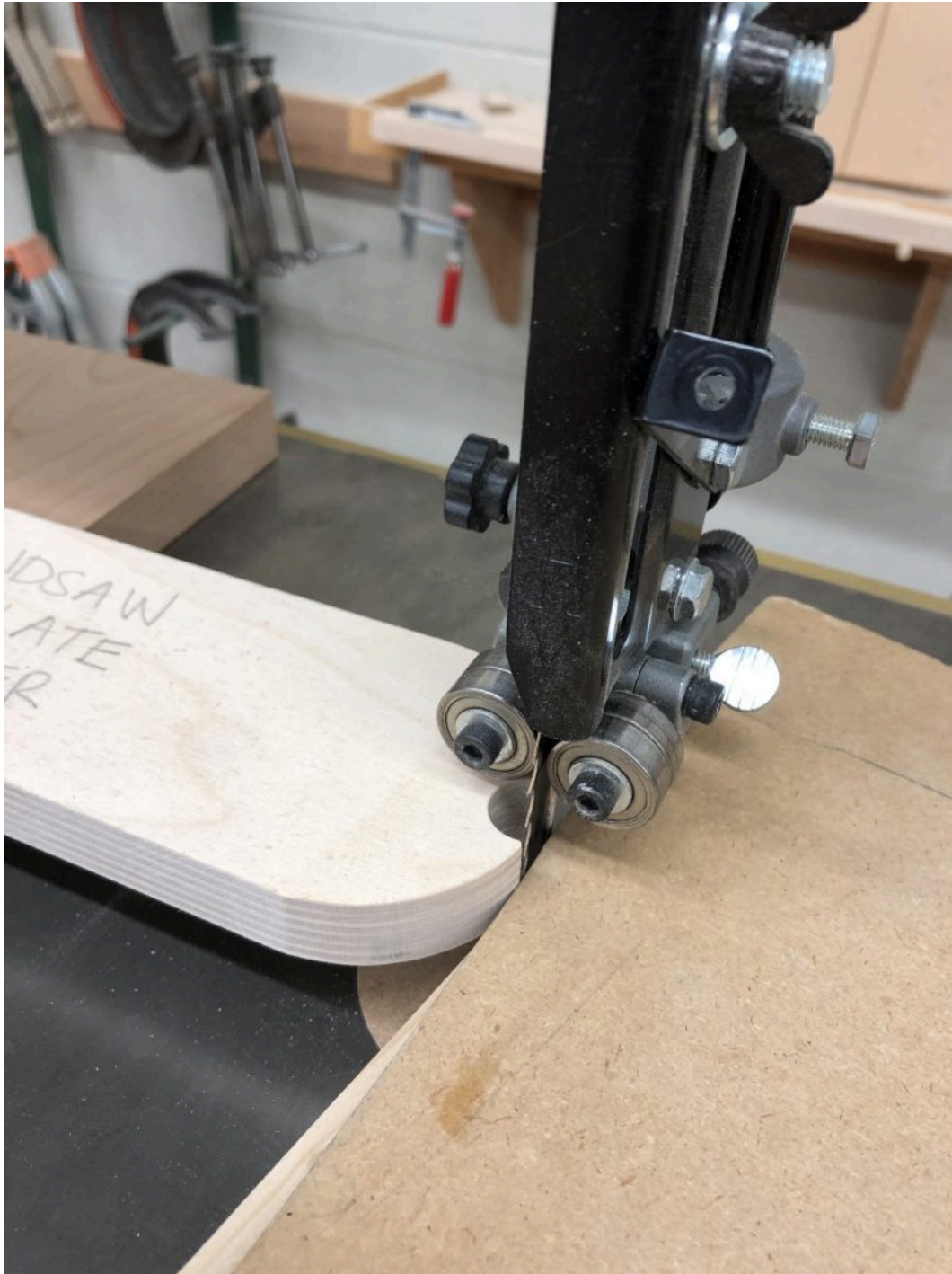
Bandsaw template follower position relative to the blade
