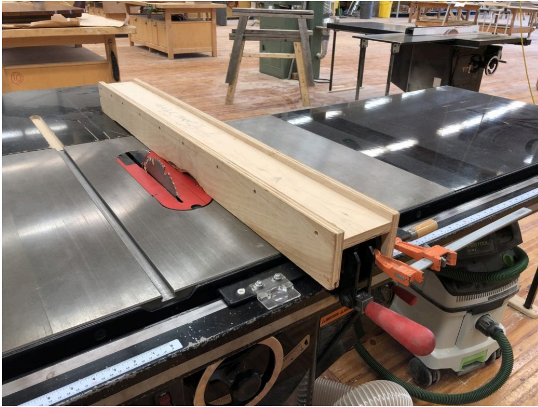
Box style zero clearance auxiliary fence
