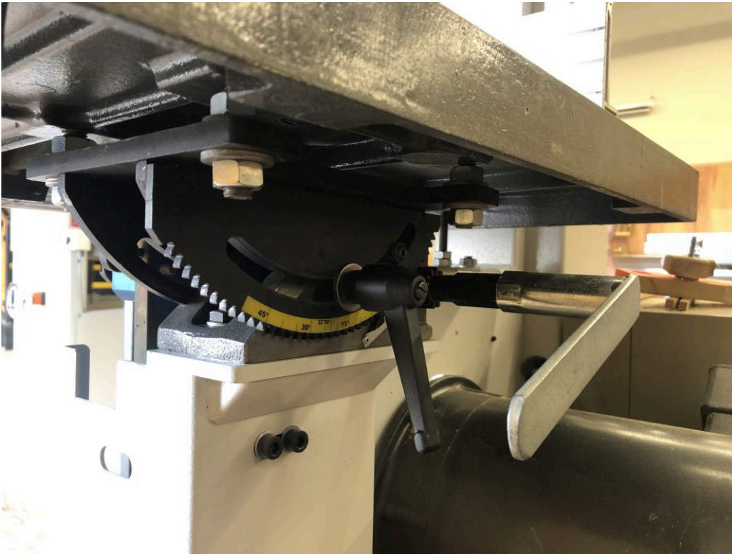
Bandsaw table tilt mechanism
