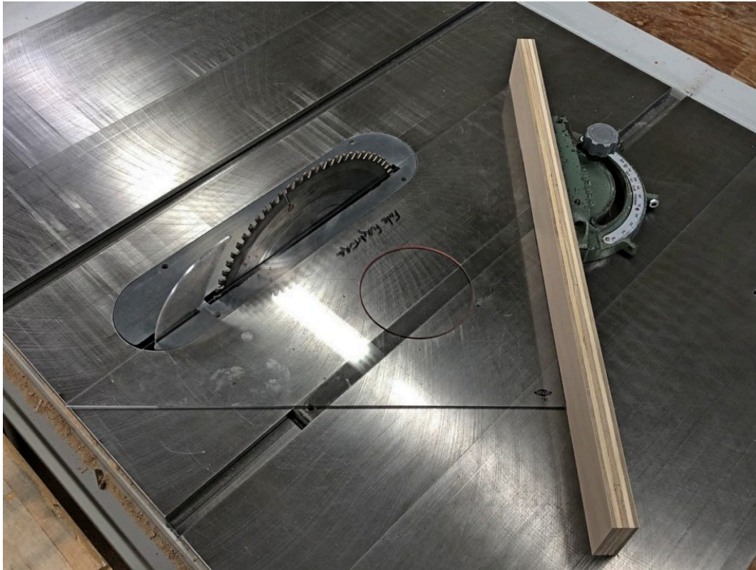
Checking the mitre gauge for 45°
