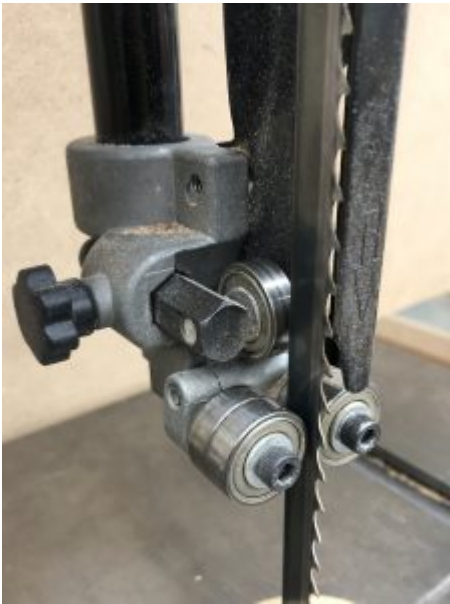
Upper bandsaw guides, bearing type
