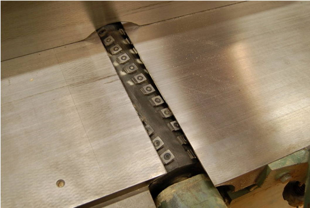
Helical cutterhead on a jointer. ***Guard removed for clarity
