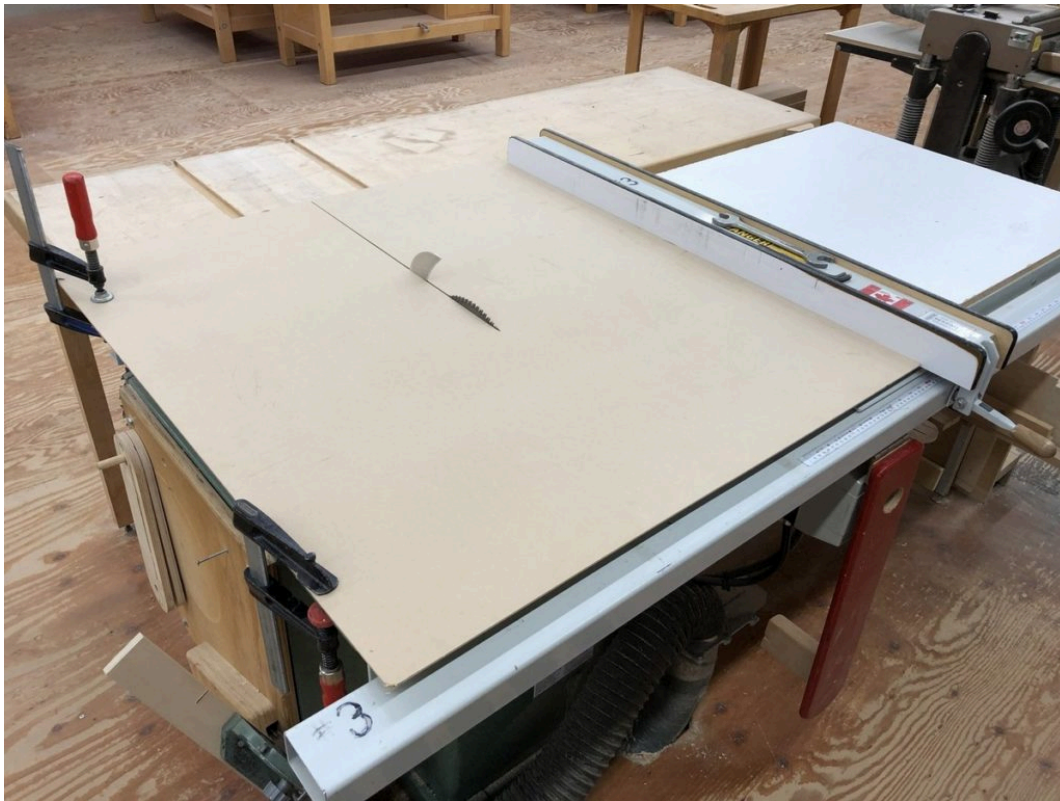
Zero clearance ripping
