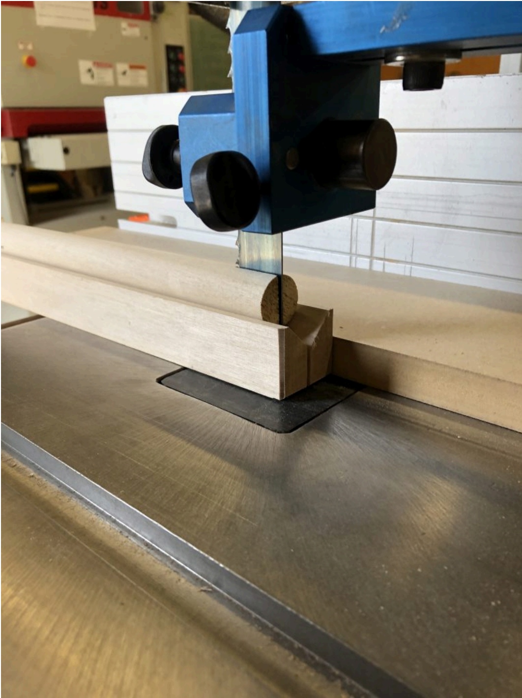
Round stock being kerfed using a V block
