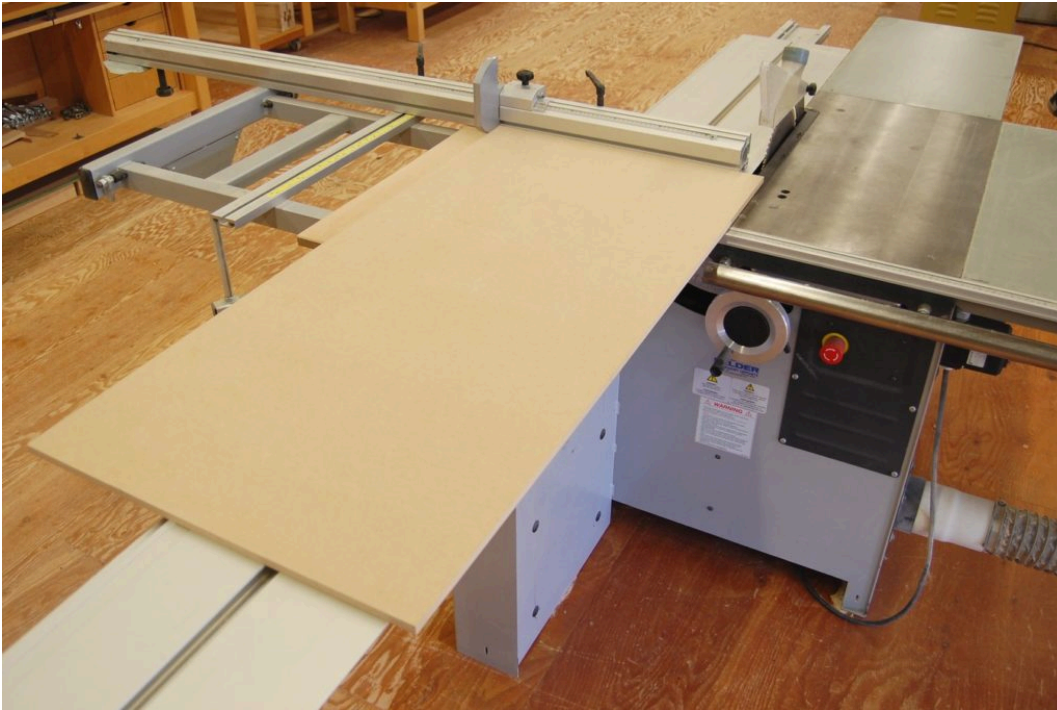
Using the crosscut fence and flip stop
