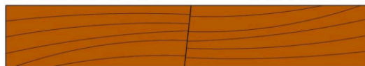
flip alternating faces, and the mating edges form a supplementary angle (straight line)
