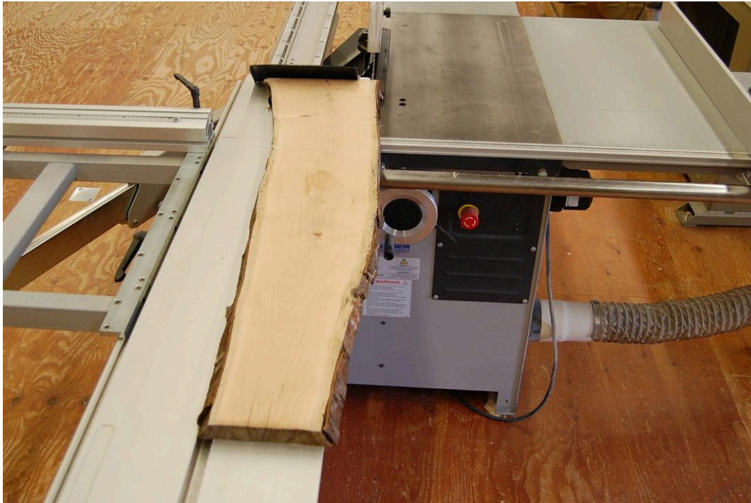
Straight line ripping on the panel saw
