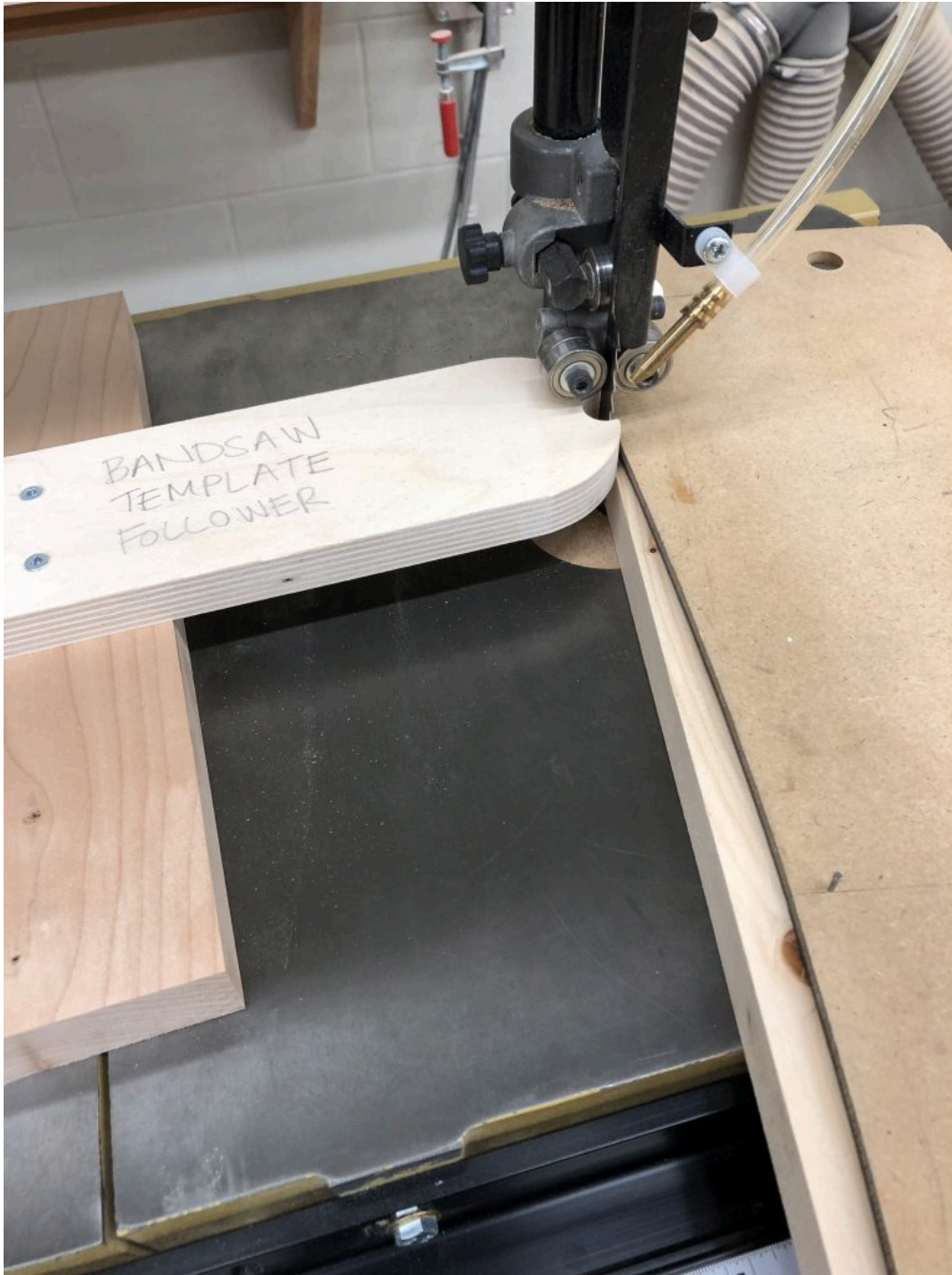
Bandsaw template follower with template and workpiece in position for cutting
