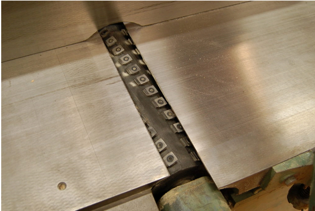
Helical cutterhead on a jointer
