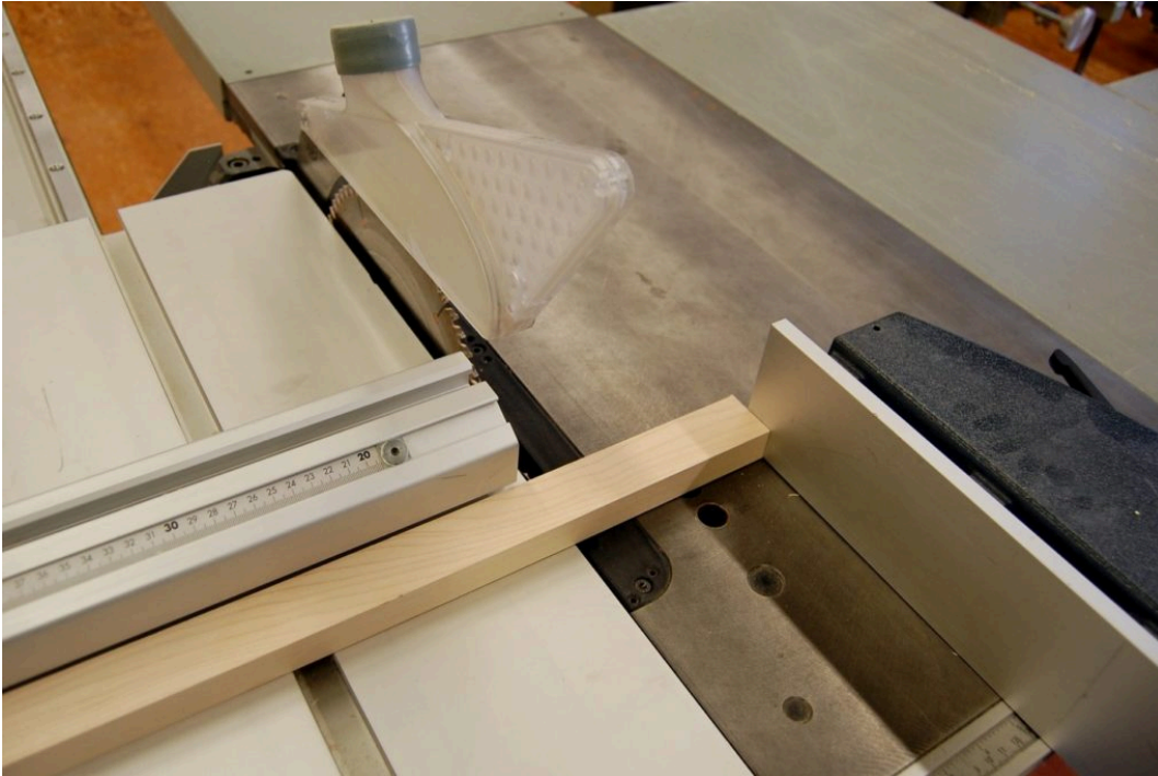
Crosscutting using the rip fence as a stop
