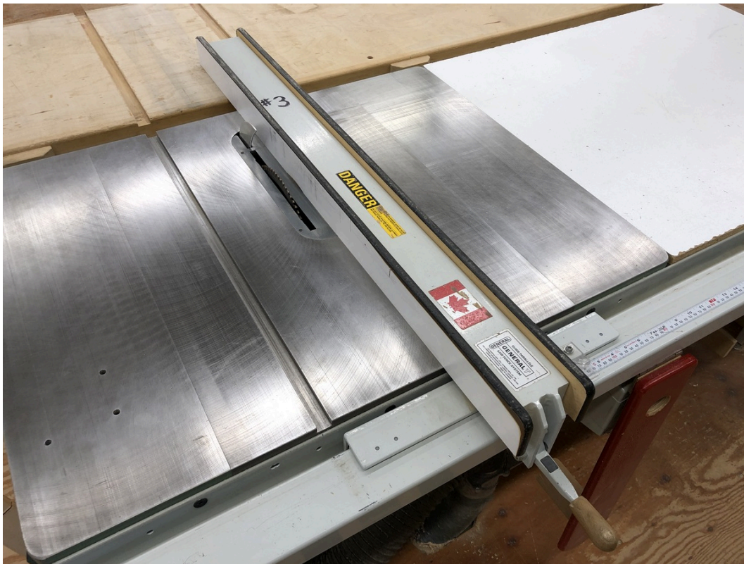
Biesemeyer "T-Square" fence installed on a 10 inch cabinet saw
