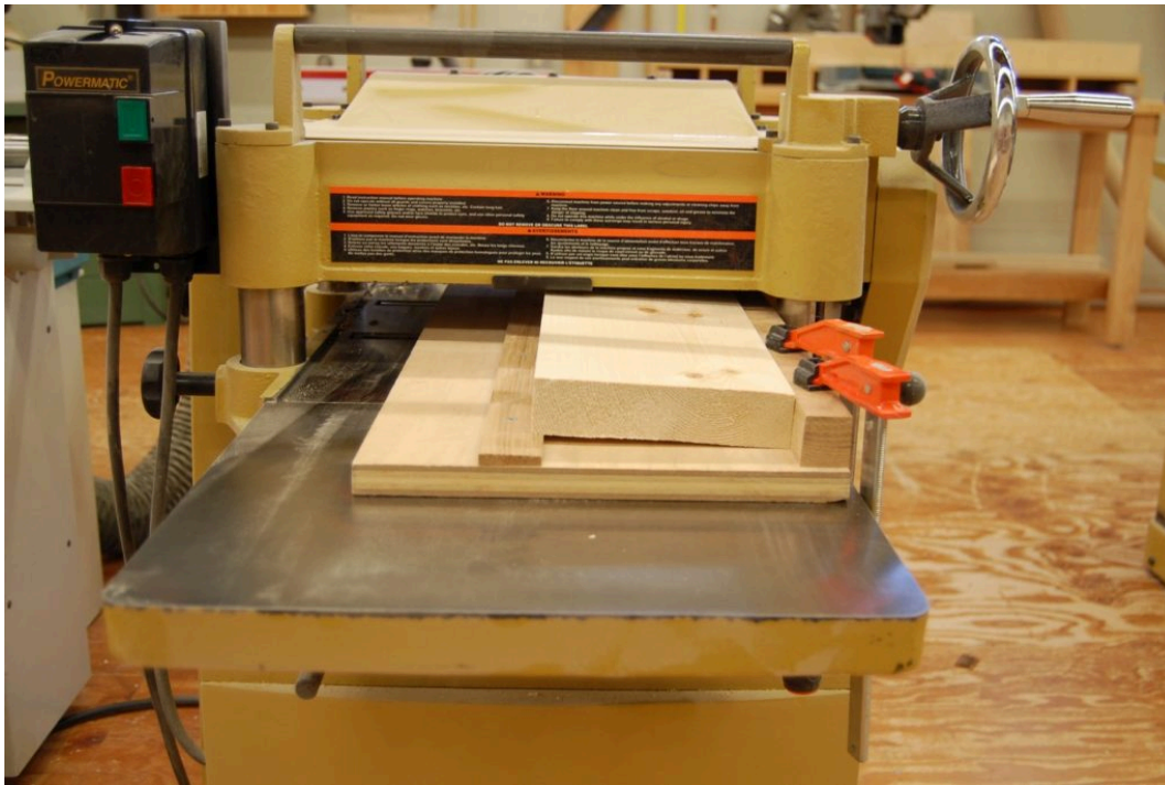
Bevel jig for the planer
