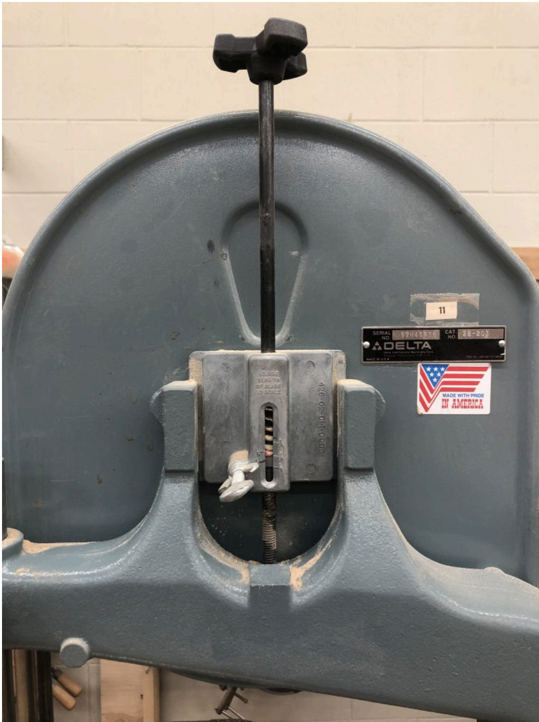
Bandsaw tension control. Note the spring visible through the slot in the square housing.
