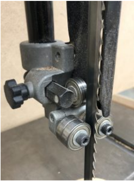
Upper bandsaw guides, bearing type
