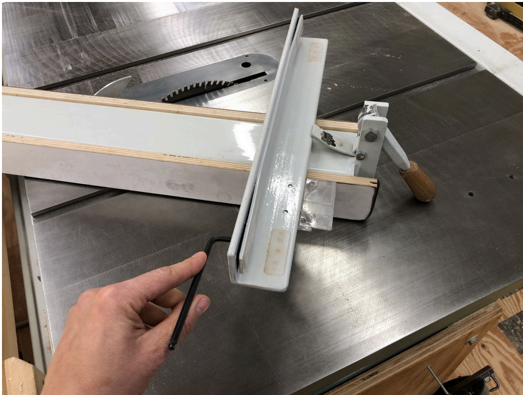
Adjusting a T style rip fence for parallel
