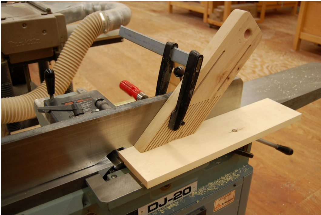
Joining a face rabbet with a featherboard
