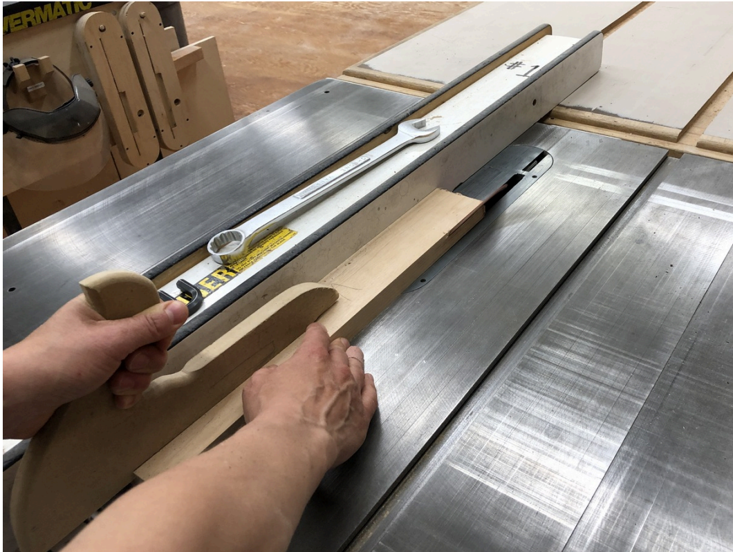
Bevel rip on a right tilt table saw. The blade is tilted at 45 degrees
