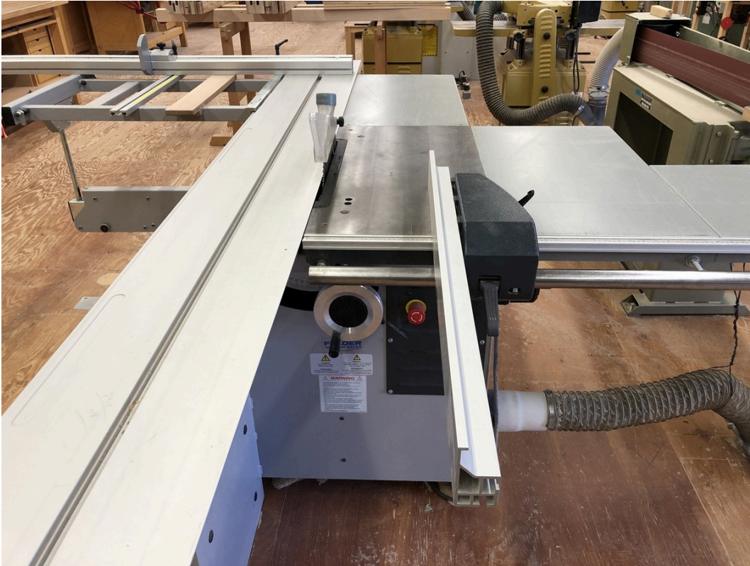
Rip fence positioned for use as a moveable stop for crosscutting.
