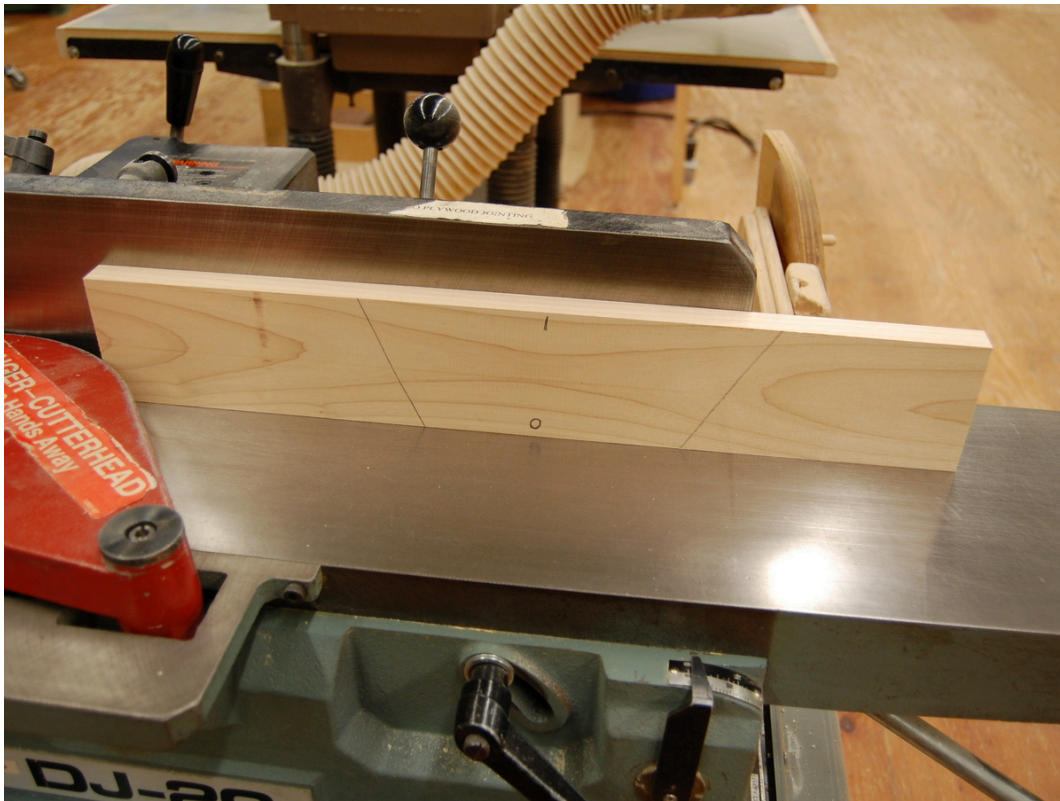
Jointing edges, face in and face out
