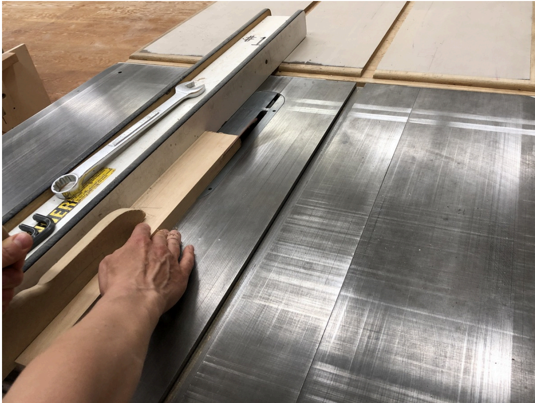
Ripping bevels on a right tilt saw
