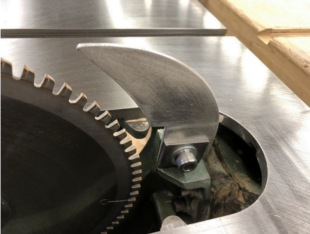
Splitter on a General 10 inch cabinet saw (throat plate removed)
