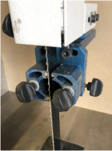
Upper bandsaw guides, ceramic type
