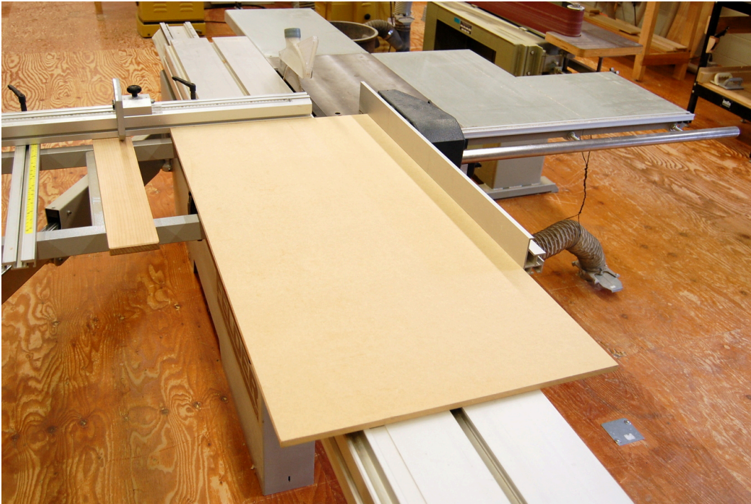
Using the rip and crosscut fence together
