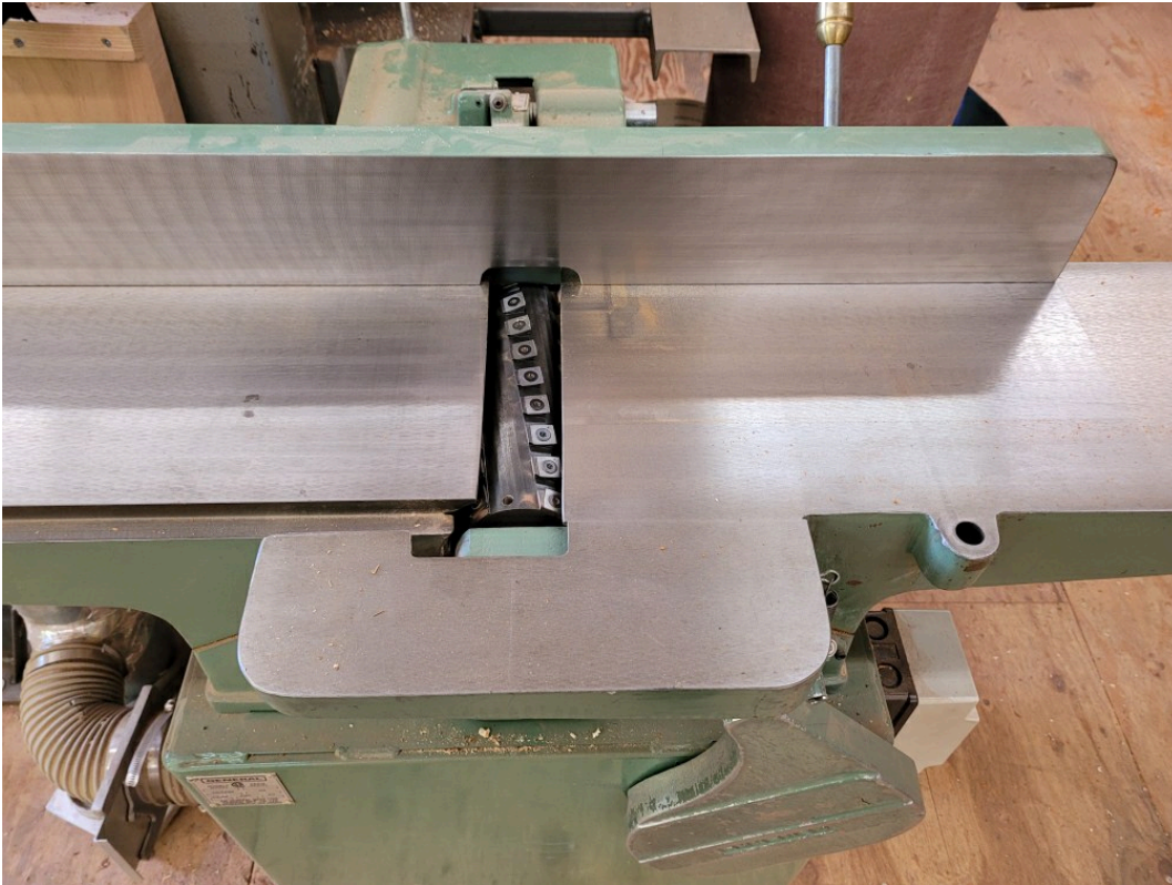
Rabbeting arm and ledge. The guard must be removed to cut rabbets.
