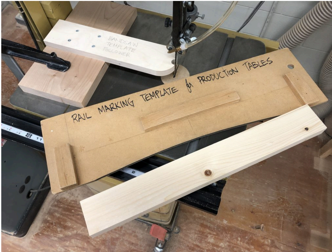
Pattern cutting follower, template and workpiece
