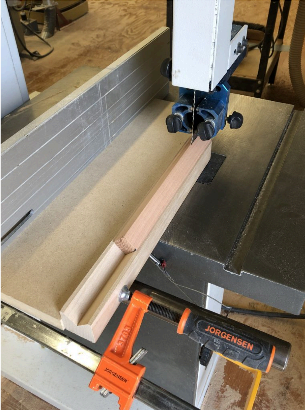
Square stock being cut in a V block. The V block is spaced from the fence to allow the guide post to be lowered to the correct height without hitting the tall rip fence
