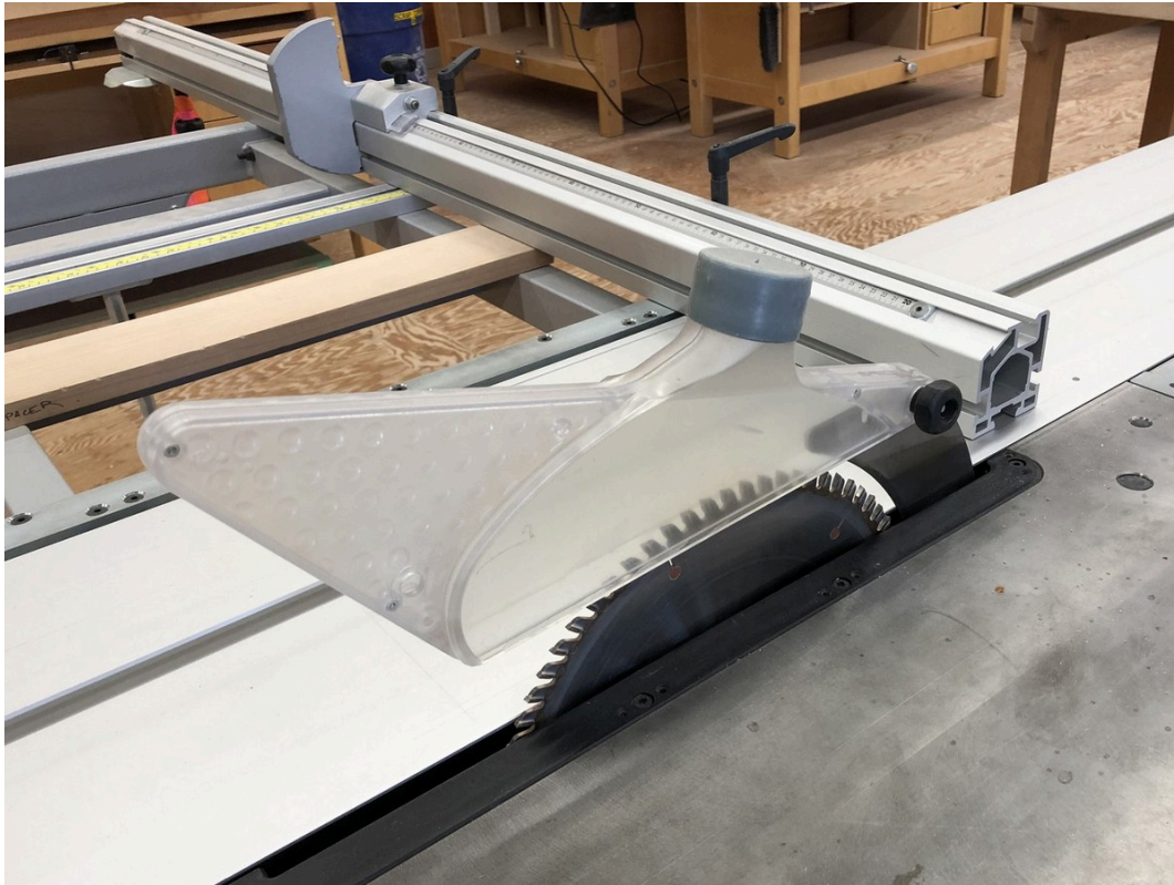
Blade guard attached to splitter on a sliding table saw
